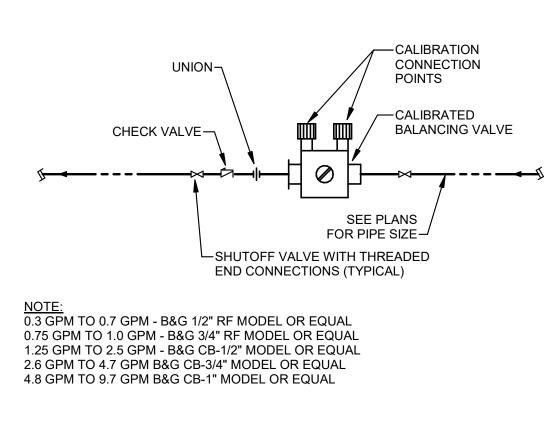
$5_{\text{NONE}}^{\text{CALIBRATED BALANCING VALVE}}$
